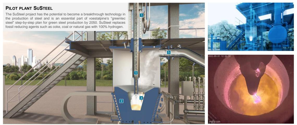
1 HYDROGEN AND IRON ORE SUPPLY Hydrogen and iron ore are fed to the plant.
