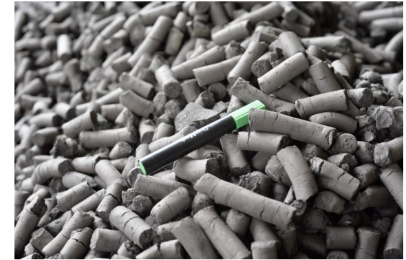
Briquettes just after production : average size 8-10 cm
