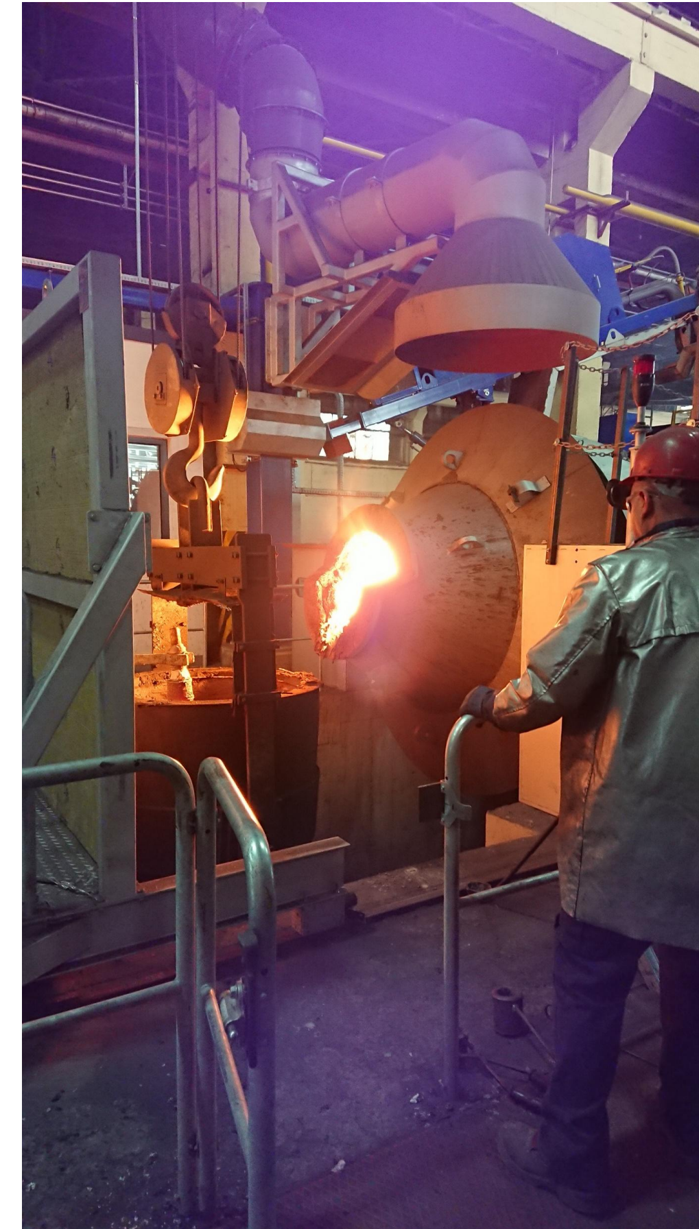
Fig. 3. Tilting the AOD converter for tapping the cast steel into the ladle
