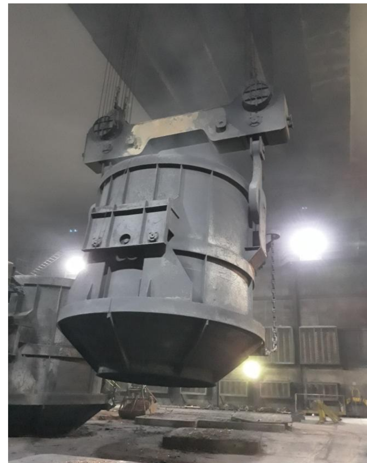
Charge basket used for loading scrap and agglomerates into the furnace. The agglomerates are placed at the bottom of the basket
