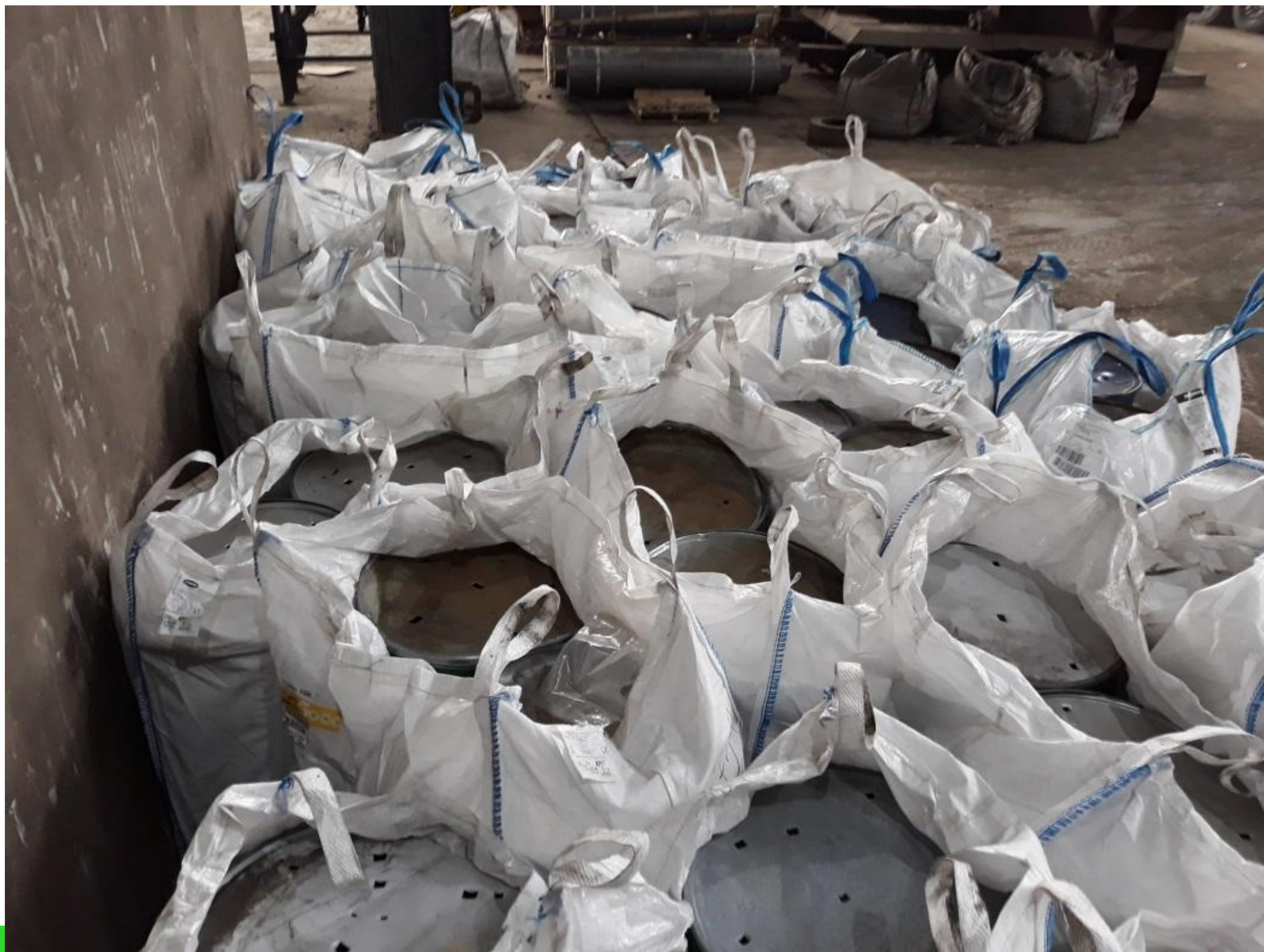
Large-size agglomerates in big-bags, prepared for loading in the charge basket
