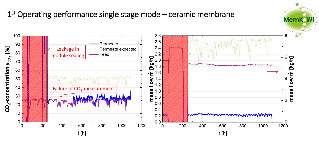
Observations: - stable operation after fixing leakage but significantly lower selectivity compared to lab-tests
