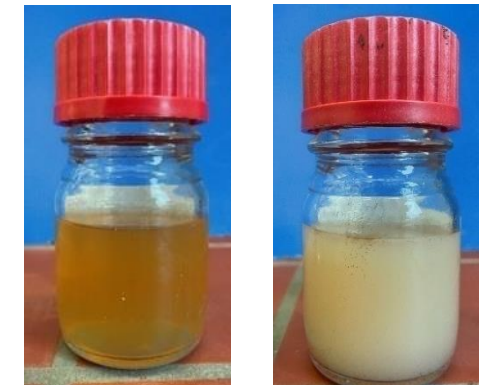
Loaded cleaning agent 6 (left) and 8 (right)
