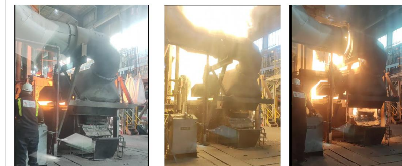
Charging briquettes and reaction in pilot plant
