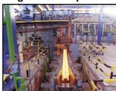
furnace before the Rolling Mill process by **using enriched air** in the natural gas burners. **Less nitrogen** that enters into the furnace means less heat losses and **natural gas savings**. The percentage of Oxygen in combustion air
