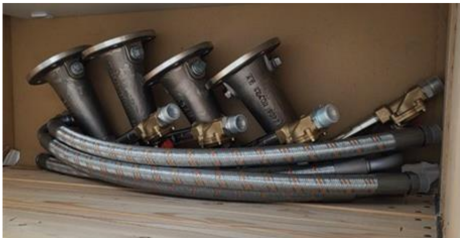
Figure 4 : AGAM horns before installation
