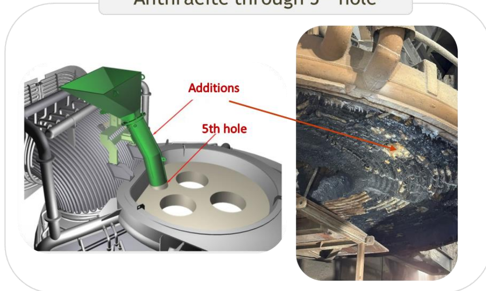
Figure 1. Anthracite added through the 5 th hole in Sidenor
