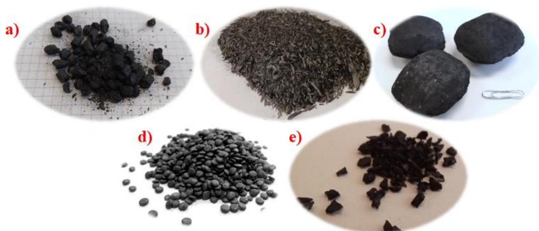
Figure 1: a), b) and c) shows different types of biochar, d) shows plastic grains; e) shows a material derived from tires.
