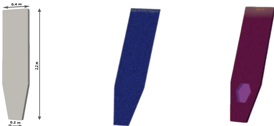
Figure 16: BFI Shaft simplified version (left), BFI shaft with pellets inside (middle) and modification with the ‘Christmas Tree’ (right)
