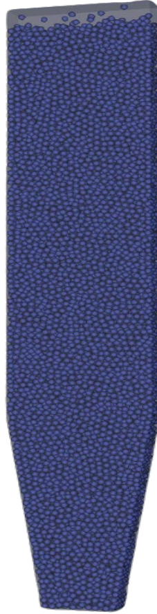
Figure 18: MIDREX Shaft Simulation for Test Cases 2 and 3 with air flowing from the bottom and particles initially placed inside the shaft geometry
