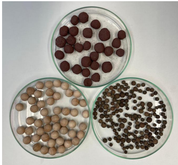
Figure 3: Sample materials used in the experiments: (top) industrial DR-Pellets; (bottom left) monodisperse wooden spheres; (bottom right) clay pellets.
