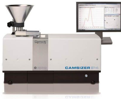
Figure 4: Camsizer for the determination of particle size and shape distribution
