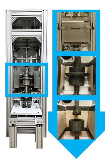
Initial tests have demonstrated that the setup is effective and can accurately simulate the flow of granular materials, such as iron pellets, under extreme environmental and stress conditions. Experiments on this setup play an important role in improving the control and efficiency of hydrogen-based steel production — a major step toward greener, low-emission steelmaking.
