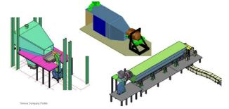
have limitations in the flow rate. The dry granulation can be conducted on-line or off-line. Tenova has different dry granulation solutions that can be adopted for specific needs for EAF or LF granulation, which result in production of amorphous materials.
