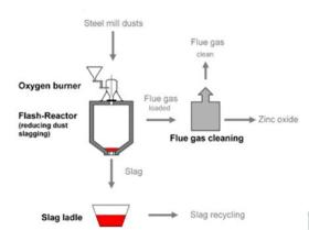
content into a slag phase, which can serve as secondary iron resource for the sintering plant or the Blast Furnace (BF). The zinc content in slag should stay below 0.5 wt.-%. For upscaling to 1,000 kg/h, a new pneumatic conveying system was installed, which uses natural gas as conveying medium.
