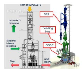
Marco Corbella and Paolo Stagnoli (Tenova) discussed the OSBF (Open Slag Bath Furnace) designed by Tenova to process low grade iron ore, while using 100% hydrogen as reducing gas. The OSBF has the same ability as a BF to run long continuous campaigns, but with higher flexibility (possibility to switch on and off). The OSBF process can produce a slag with the same or better quality then other furnaces resulting in a material, which can be valorised in concrete, cement, mortar or as aggregates.
