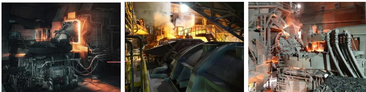
Figure 20: Top charging of hydrochar pellet at EAF (150 t) of Pittini, Italy (left), top charging of hydrochar/mill-scale briquettes at EAF (85 t) of ORI Martin, Italy (middle) and hydrochar injection trials at EAF (150 t) of CELSA, Spain (right).
