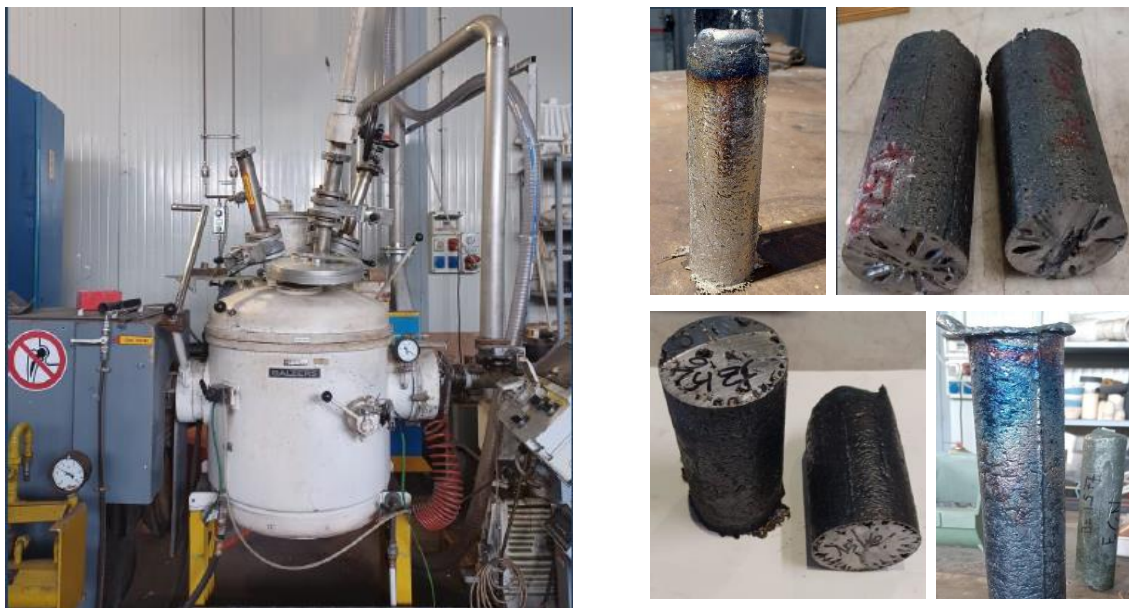
Figure 3: BALZERS VSG 10 vacuum induction furnace (left) and examples of cast ingots after hydrochar addition to liquid iron (right).
