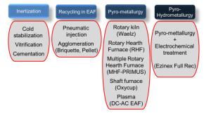
Figure 14: Dust treatment process
