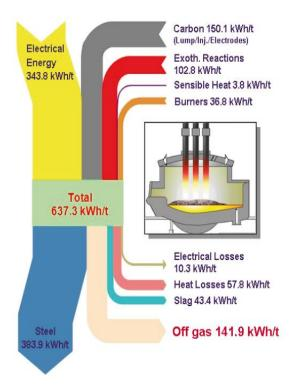
Figure 19: EAF Sankey diagram [A-P Hollands et al., METEC, Düsseldorf, 27 June – 1 July 2011]
