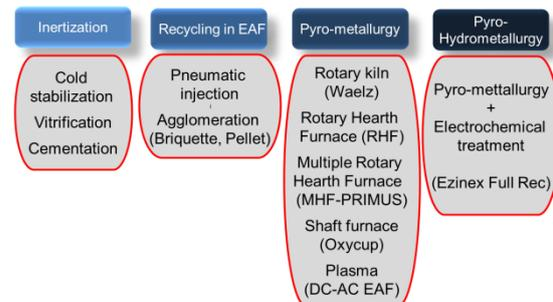
Figure 14: Dust treatment process
