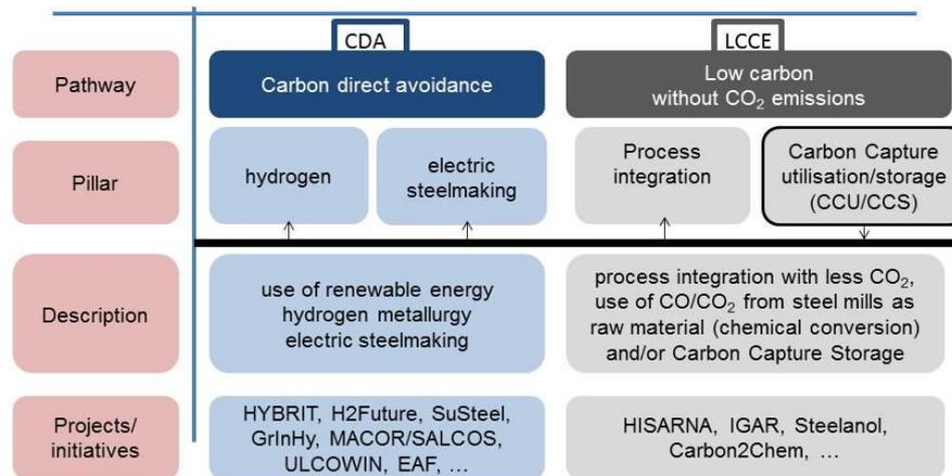
Figure 20: Two pathways in low-carbon projects (Big Scale)
