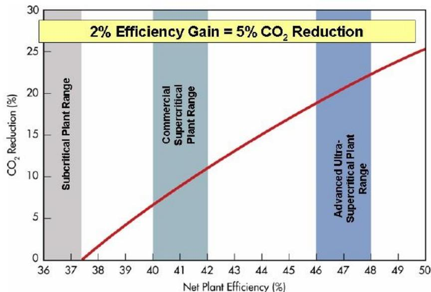
Figure 29: Efficiency improvement for advanced USC fossil power plant
