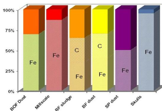
Figure 11: Iron & steelmaking residue
