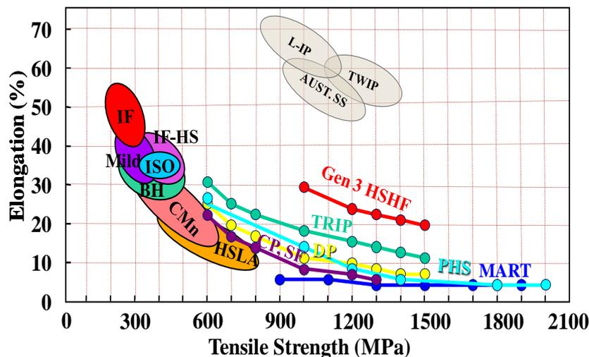
Figure 2: Range of mechanical properties of various steel grades
