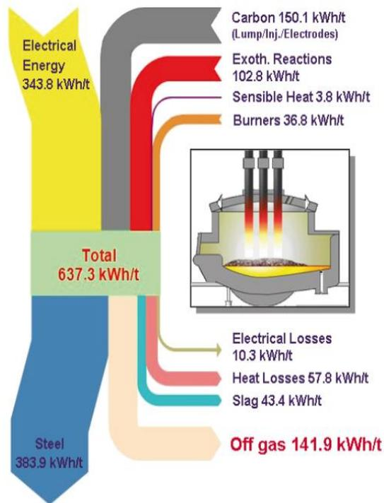
Figure 19: EAF Sankey diagram [A-P Hollands et al., METEC, Düsseldorf, 27 June – 1 July 2011]
